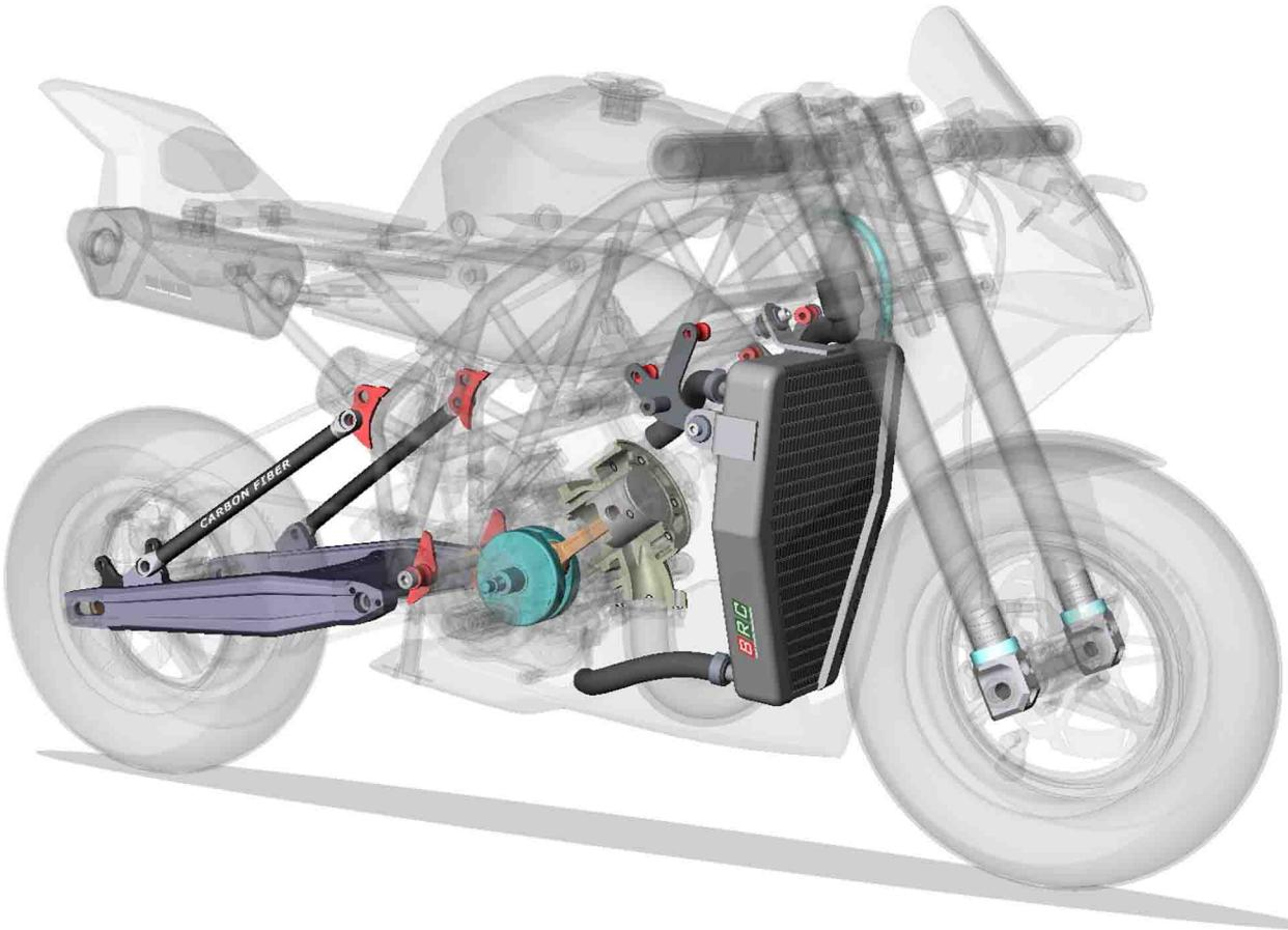
*The new rear fork, XL radiator, adjusted crank and cylinder, better engine balancing and performance, new engine mount in the frame and upgraded geometry of the chassis are the main features of the Ultima minibike 2010. Apart from these main characteristics, Ultima can offer lots of other little upgrades and innovations. As usual, minibike Blata is low-weighted and offers great bike handling.*
